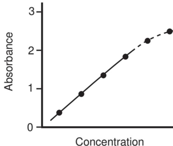
The most reliable measurements are obtained when  $0.1 < A < 1$
