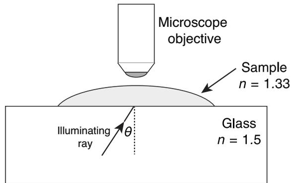
The key element is a glass block through which illuminating light rays pass at an angle set to produce total internal reflectance between the glass and the sample above it. The indices of refraction for the glass and sample are indicated in the drawing.
